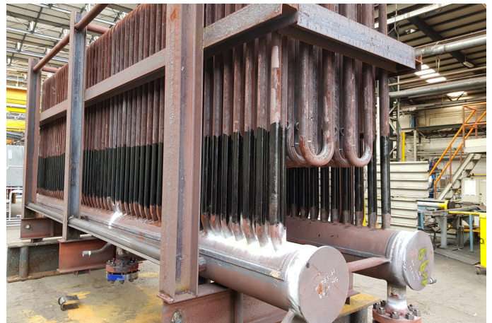
Water-based epoxy coatings for high temperatures on heat exchangers
